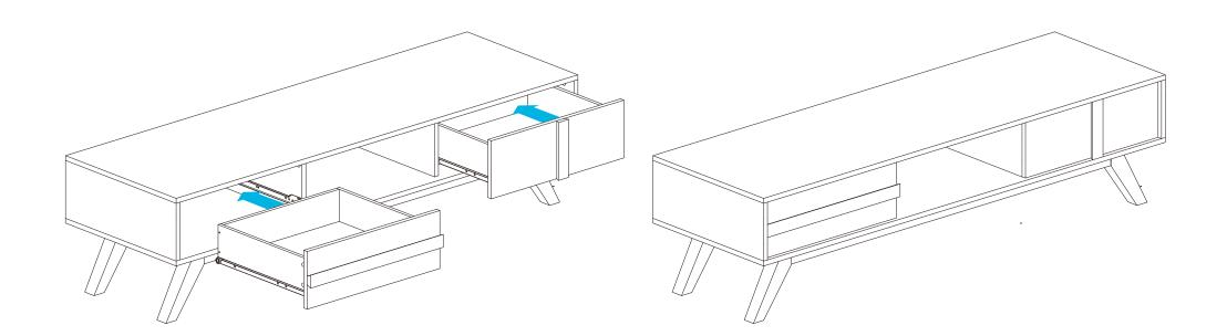
Flip the side board unit over onto its legs. To complete the assembly slide both completed drawers into place on the rails in the side board unit as shown.
