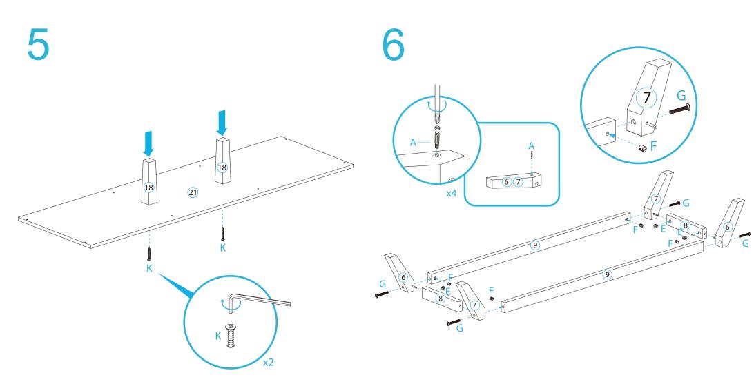
Attach the two central legs [18] to the base panel [21] using 2x screw bolts (K) through the underside and tighten with allen key (L) provided.
