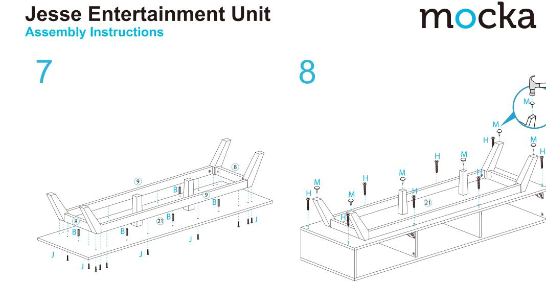
Attach panel [21] to leg panels with 8x dowels (B) and secure with 20x screws (J). Tighten with a screwdriver.
